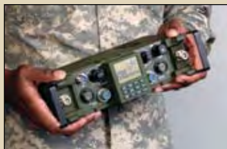
Figure 3 JTRS HMS radio product lines allow individual warfighters to have networked communications capability, enabling coordinated joint force and coalition operations. Shown here is the Manpack form-factor.
